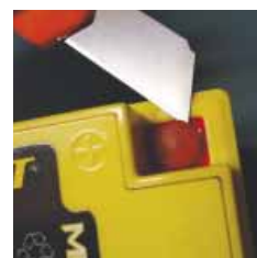
Removal of terminal plugs
