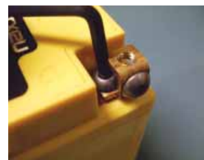
Attaching the terminals
